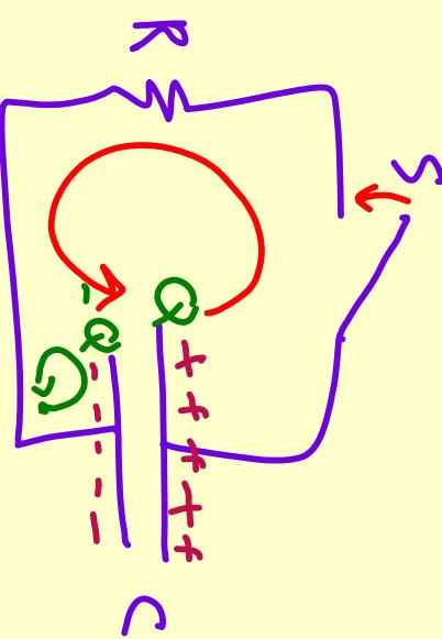
$$\int_{0}^{t_1} \frac{-\frac{dq}{dt}}{RC} dt = \int_{Q_0}^{Q_1} \frac{dq}{C}$$
