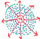
flux through the surfaces is independent of the radius  $r_1, r_2, \dots, r_n$  of the Gaussian surface. (4)
